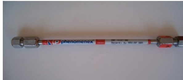
Resim- 3: Kolon; synergy 4 \mu , MAX-RP 80 A, 150 x 2.00 mm, 4 micron
