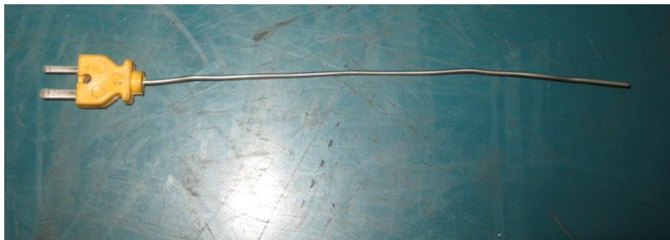
Figure 3.5. Thermocouple which is located inside the p.plate
