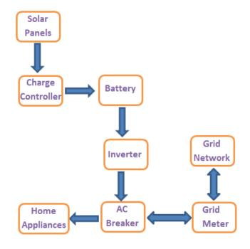
*Figure 7:* Setup diagram of the system
