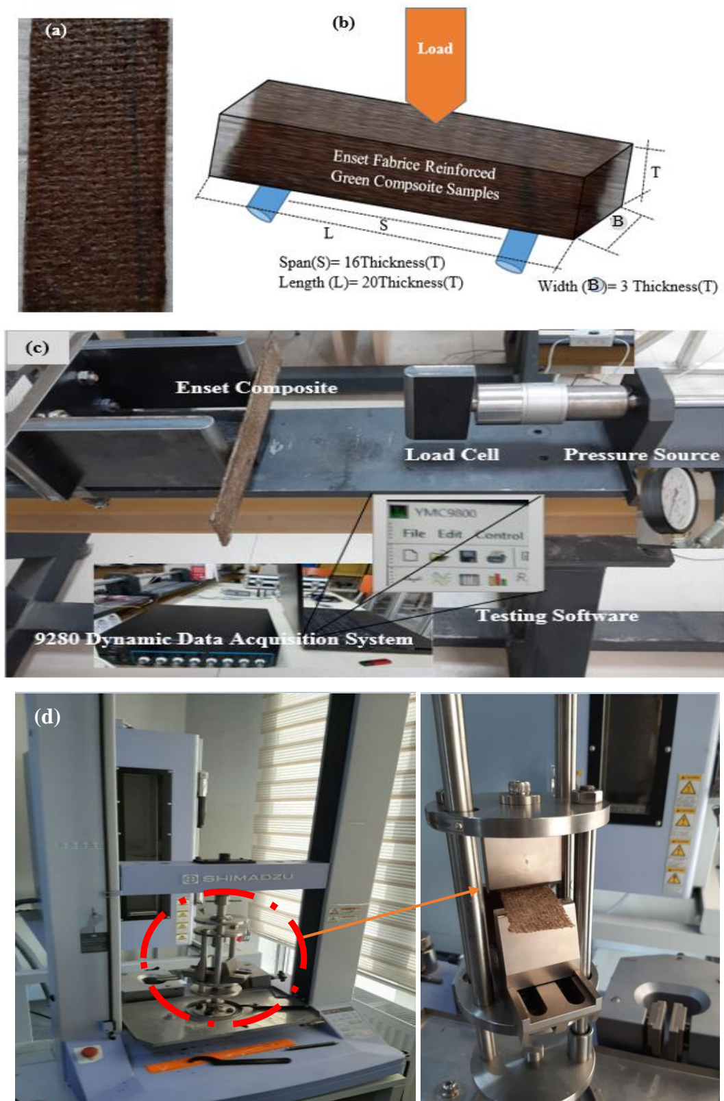
Figure 3.11. a) Enset fabric reinforced composite specimens b) Schematic illustration of 3 point bending flexural test c) Dynamic flexural strength tester d) Shimadzu strength tester
