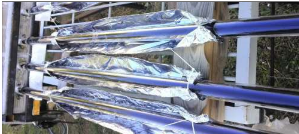
Figure 4.31. View of placing the reflector around the glass tubes
