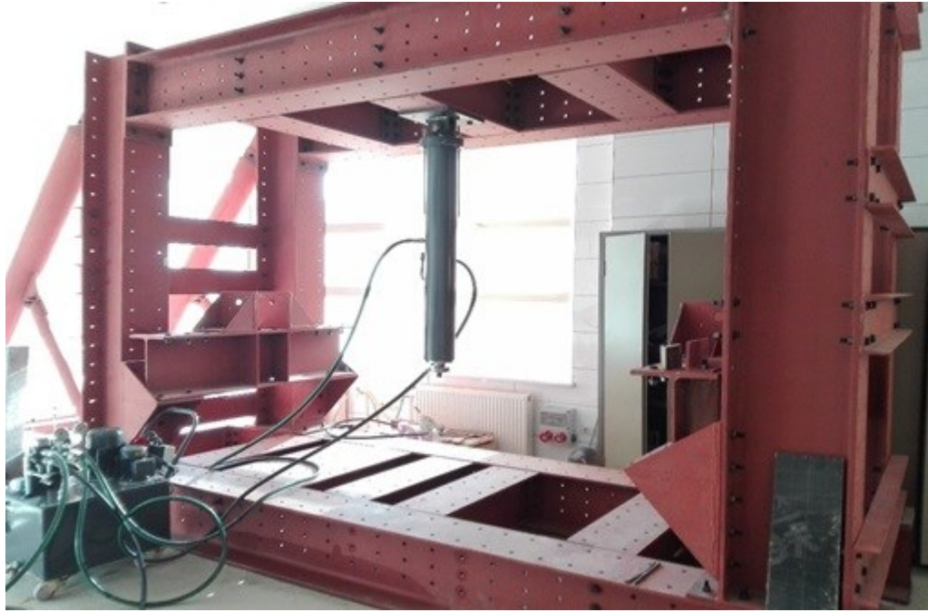
Figure 3.6 Demonstration of the loading system and the hydraulic piston used
