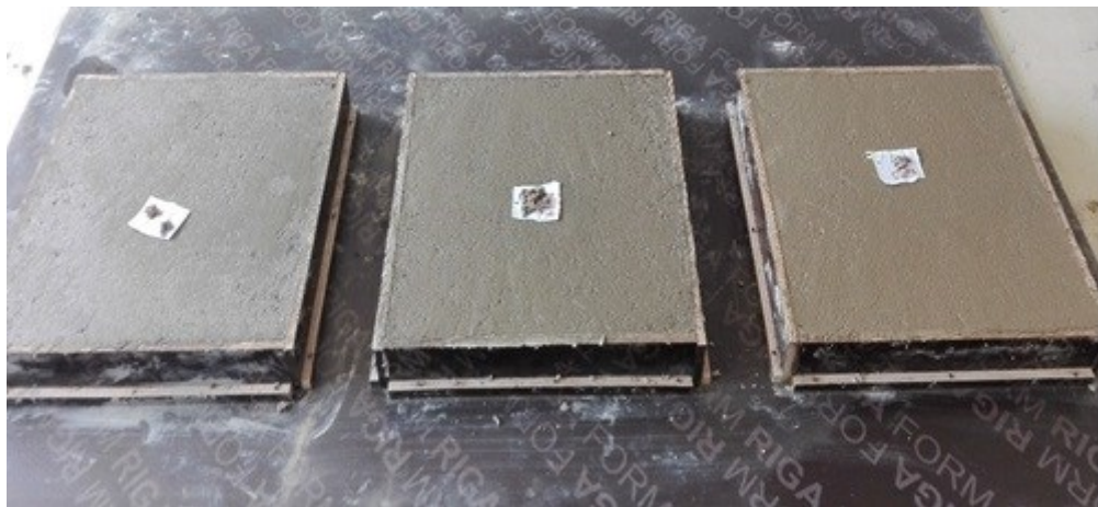
Figure 3.9 Concrete samples in plywood mold.
