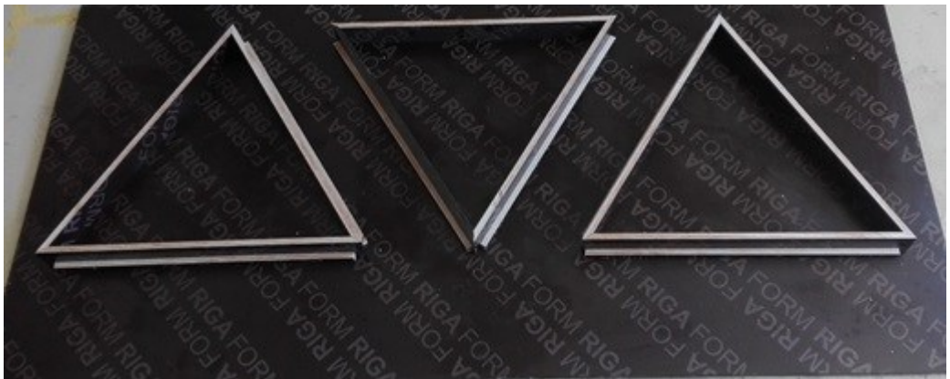
Figure 3.3 Triangular panels mold -800 mm.
