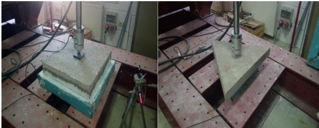
Figure 3.10 The two types of test Square panel & Triangular panel test
