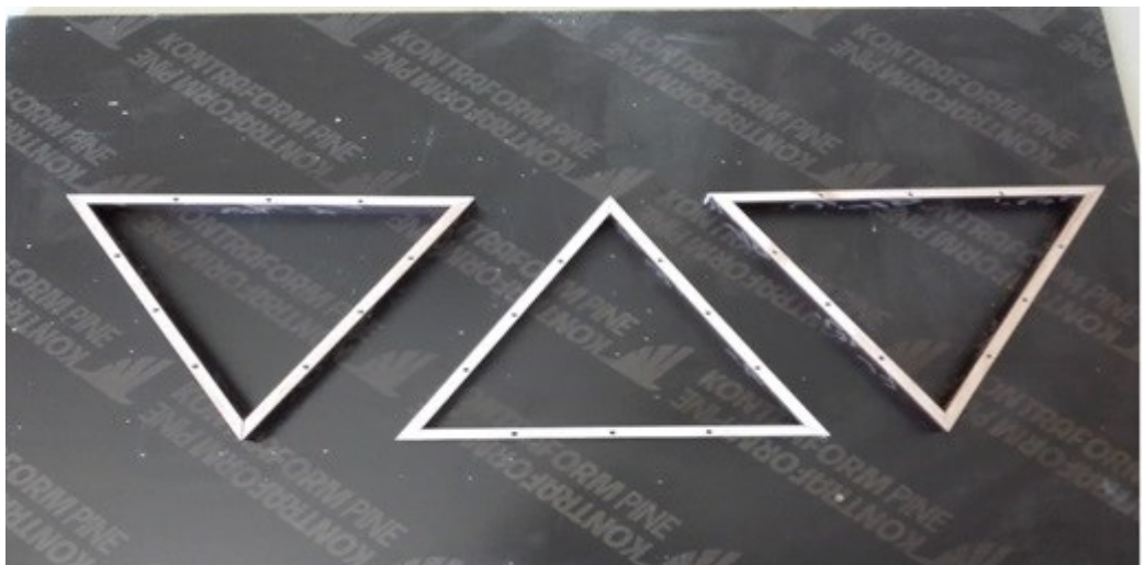
Figure 3.4 Triangular panels mold -500mm.
