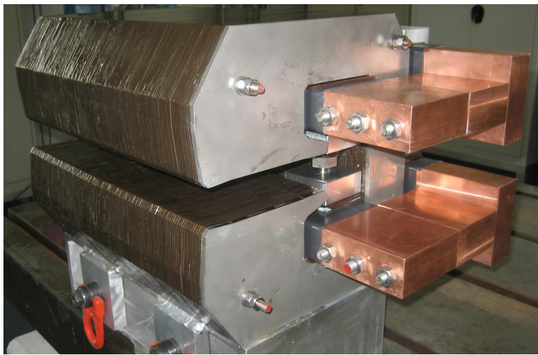
Figure 8.8: One of the 400 mm long model magnets made at CERN with interleaved laminations.
