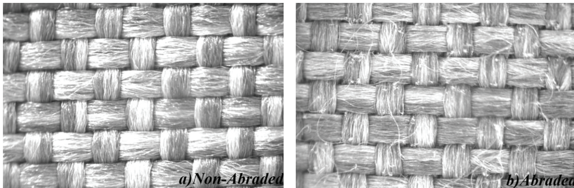
Figure 6. A microscopic view of F2 fabric a) before and b) after 20000 cycles of abrasion
