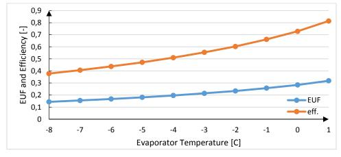
Figure 7: The influence of the evaporator temperature on EUF and system efficiency  $(\eta_{PT})$
