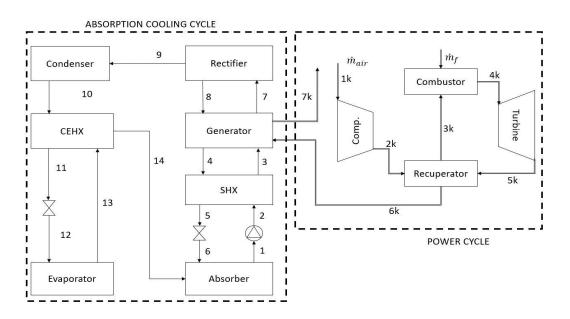
Figure 1: Scheme of the combined microturbine-NH<sub>2</sub>/H<sub>2</sub>O absorption cooling system
