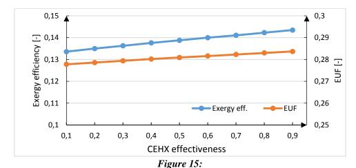
The influence of the refrigerant heat exchanger's effectiveness on the exergy efficiency of the chiller and the EUF
