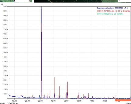
Figure 19 Diffractogram of the sample T-4(S B-2 en).
