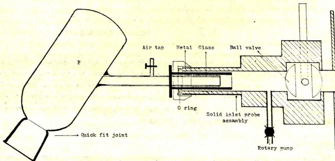
Figure 3 — Coupling unit for 2001 GC-MS TOF mass spectrometer
