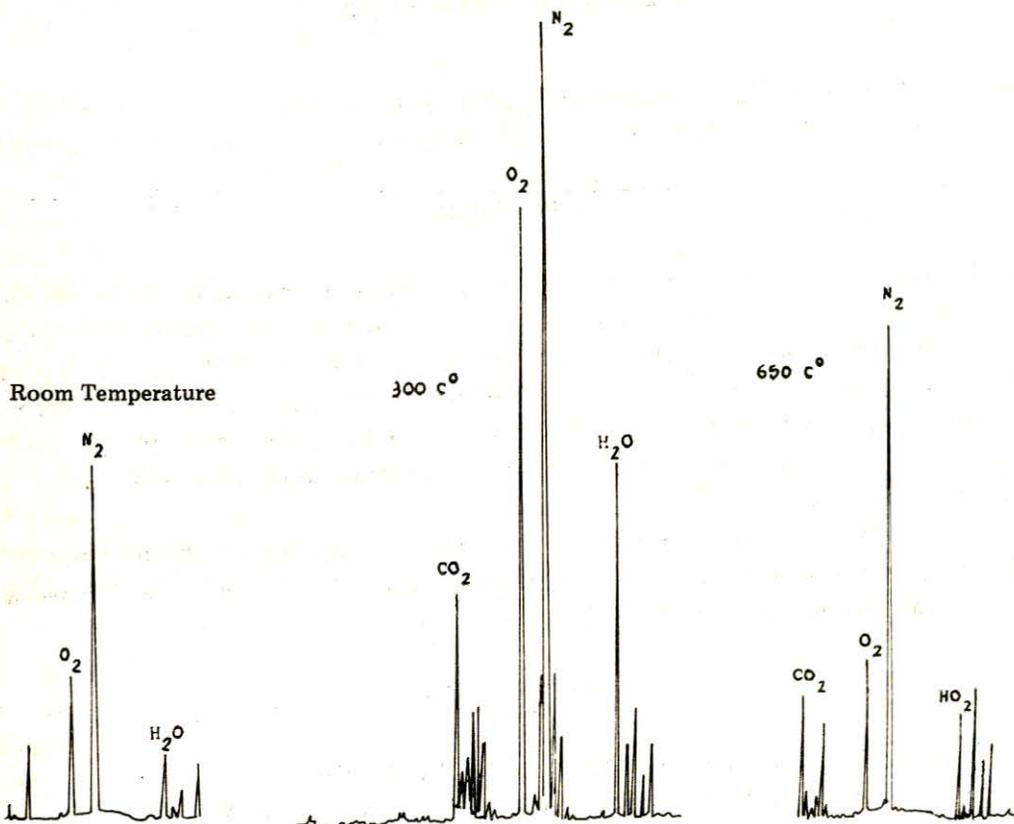
Figure 4 — Mass spectrum of the natural CaF<sub>2</sub> in the annealing process
