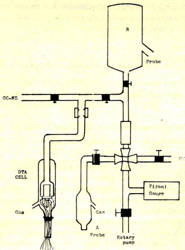
Figure 2 — Gas and volatile liquid inlet system of 2001 GC-MS TOF mass Spectrometer
