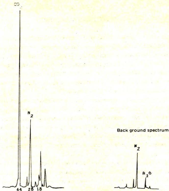
Figure 5 — Spectrum of CO<sub>2</sub> gas
