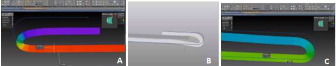
Figure 4.21. Quick Hemming Spring Back Effect Analysis Results.
