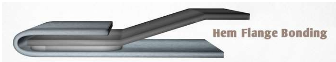
Figure 3.1. Applied sealer between the inner and the outer panel.
