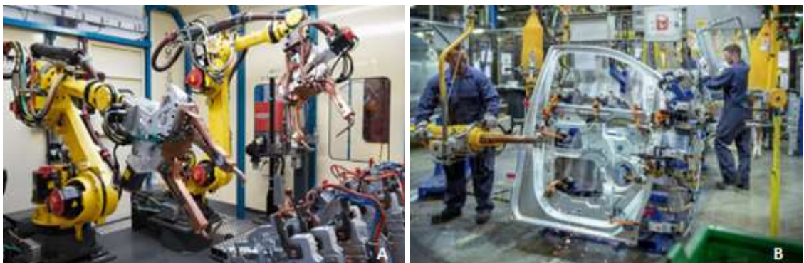
Figure 2.6. A) Robotic welding. B) Manual welding.
