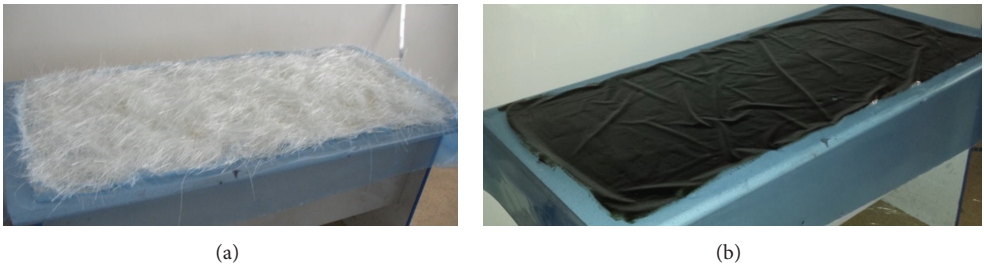
FIGURE 1: Prepreg formulations containing (a) CaCO 3 and (b) basalt particles.
