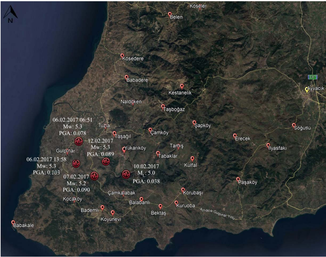
Figure 9: Villages affected by Ayvacik earthquake swarm and locations of investigated earthquakes
